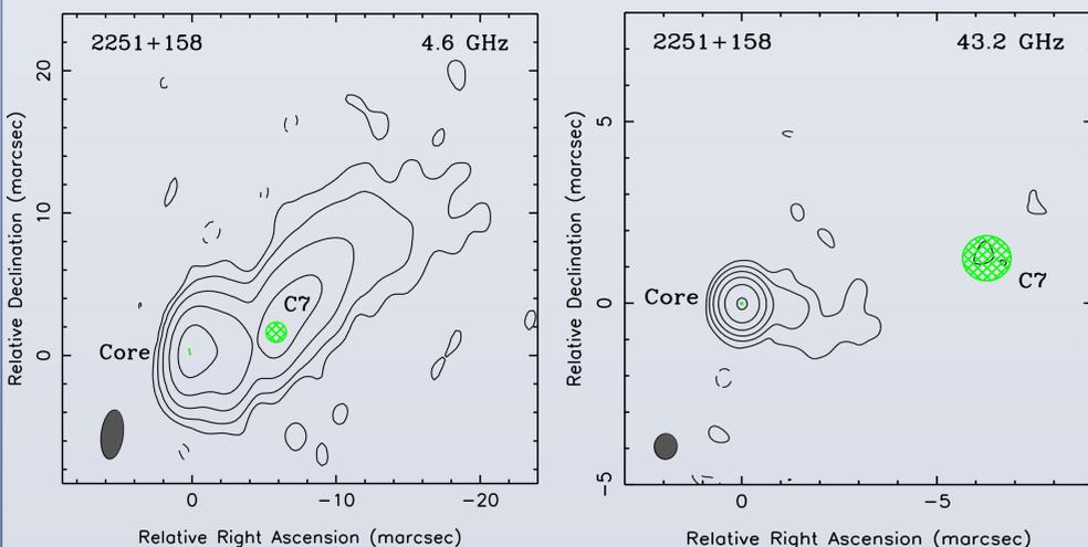
Fig 1. Naturally weighted total intensity CLEAN images of 3C 454.3. The image peaks are 3.3 and 23.5 Jy/beam for the 4.6 and 43.2 GHz image, respectively. The contours starting at 6 mJy/beam are a factor of 4 apart for all images. The beam is plotted in the lower left corner of each image.
